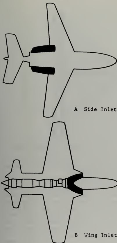
FIGURE 2-20. Two types of divided-entrance ducts.
